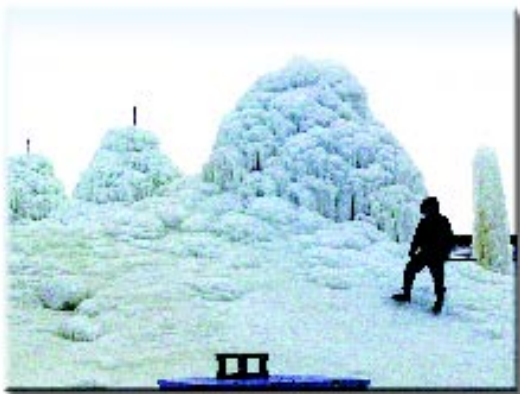
Successful field tests of the EERC's freeze-thaw/evaporation process have been conducted in New Mexico, Wyoming, and
