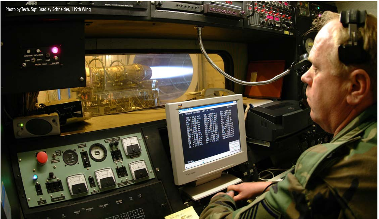
Master Sgt. Ronald "Rocky" Brovold, of the 119th Maintenance Squadron propulsion element, operates controls of an aircraft engine test facility, better known as the hush house, March 29, 2001 at the N.D. Air National Guard Base. Brovold was conducting a full-throttle analysis of a Pratt and Whitney F-16 engine to verify performance.
