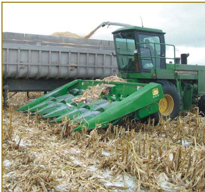
Figure 2. Harvesting snaplage in northeastern North Dakota using a self-propelled forage harvester and a snapper head.
