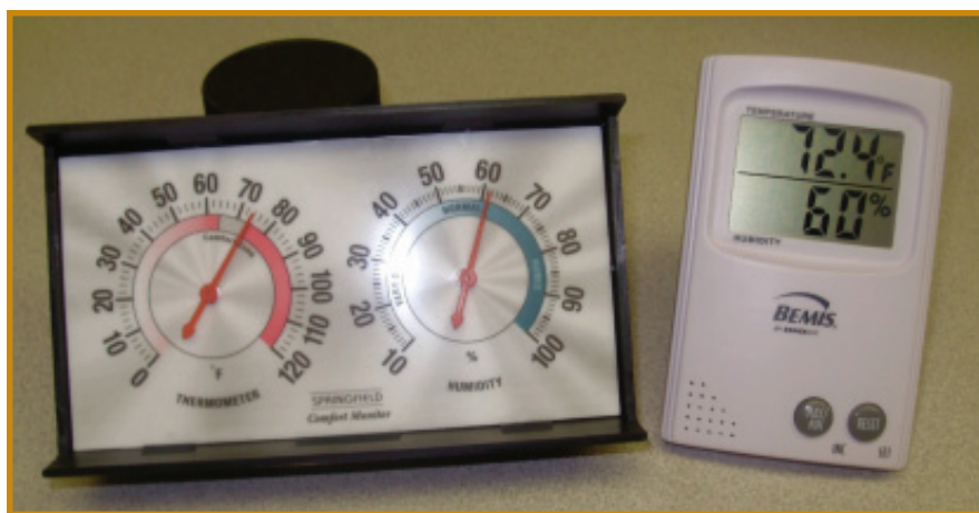
Figure 1. Examples of relative humidity meters, also known as hygrometers. (Photo by Carl Pedersen)
