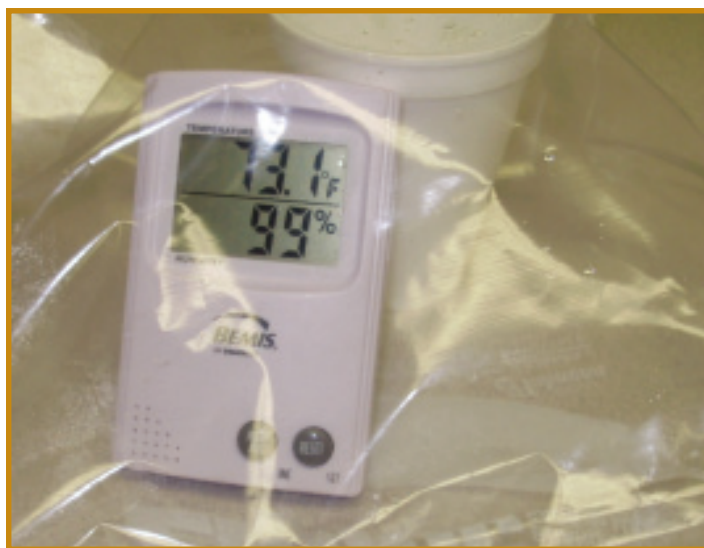
Figure 2. Calibration test, 100 percent humidity. (Photo by Carl Pedersen)
