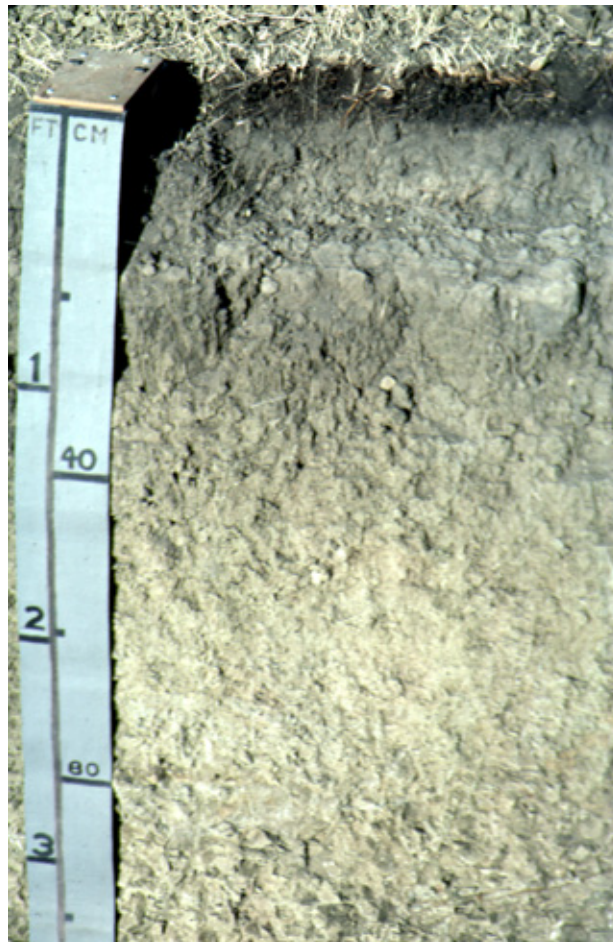
Figure 2. Profile of Janesburg silt loam. The dark brown and gray surface layers are underlain by a brown, dense, sodium affected subsoil.
