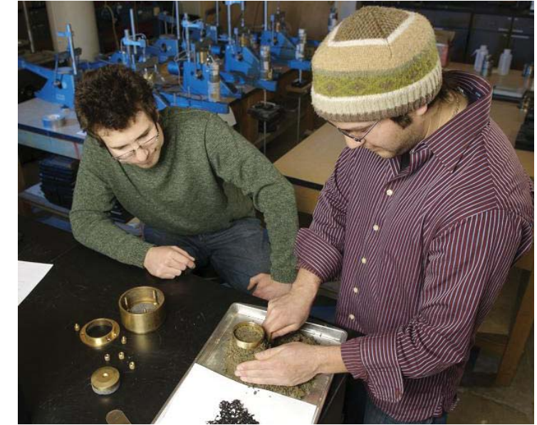
Research assistants Gabriel Iltis (left) and Jesus Higuera Seda (right) working on the preparation of specimens of expansive soil-rubber (ESR) mixtures for swell-consolidation testing.
