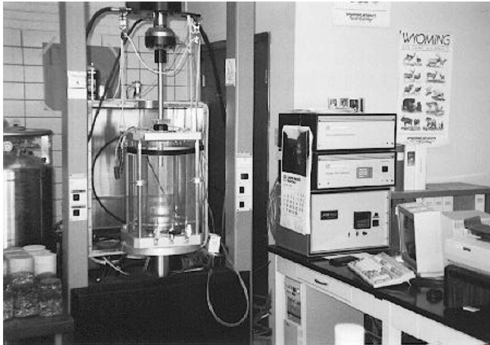
Figure 3.4 Interlaken Resilient Modulus Testing Equipment
