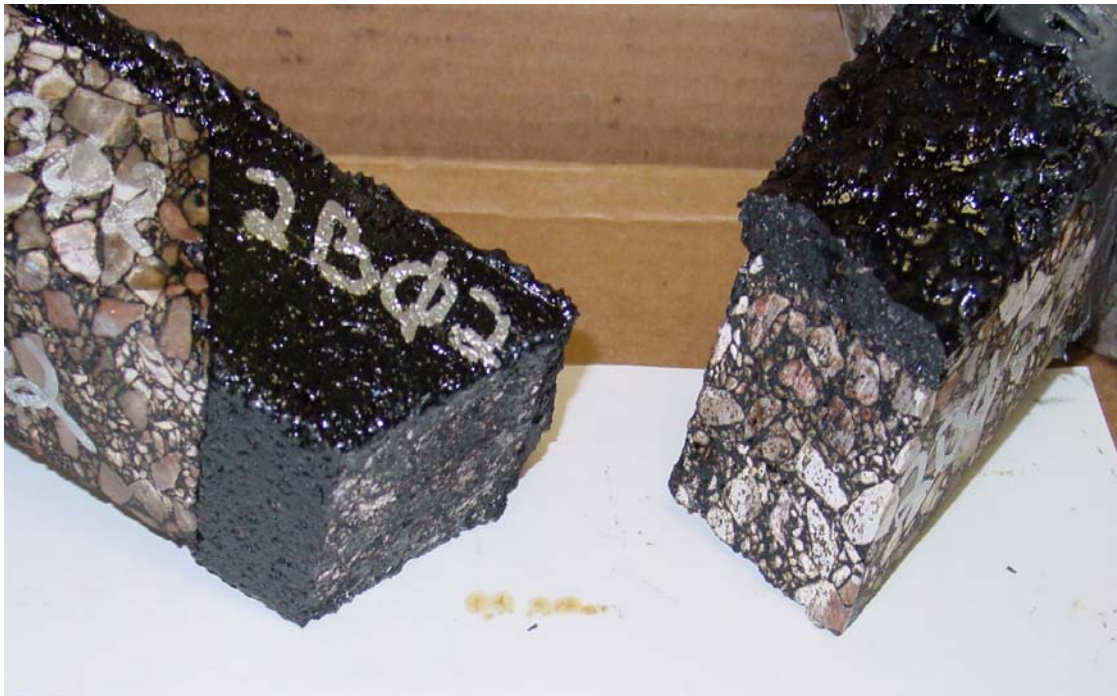
Figure 5.8 TSRST Overband Configuration Failure Mode for All Materials
