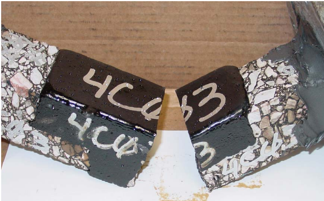
Figure 5.11 TSRST Mill & Fill Configuration Secondary Failure Mode for All Materials
