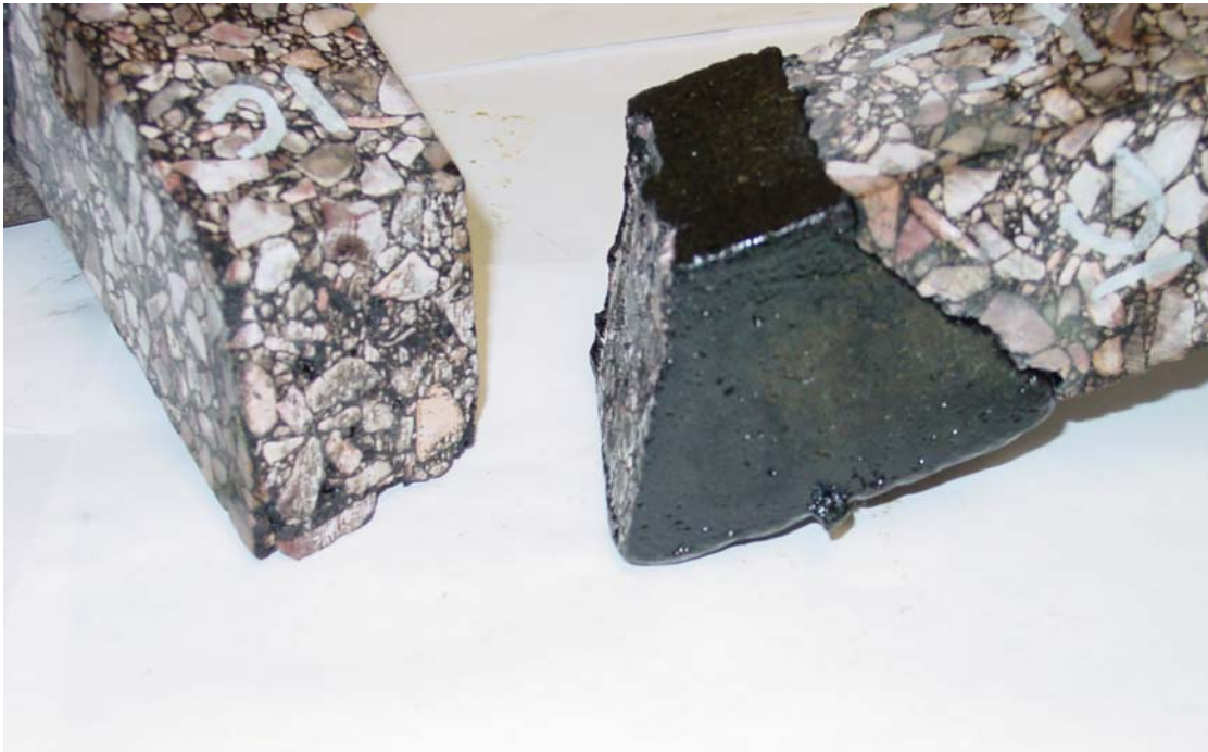
Figure 5.7 TSRST Flush Configuration Failure Mode for All Surfacing Materials
