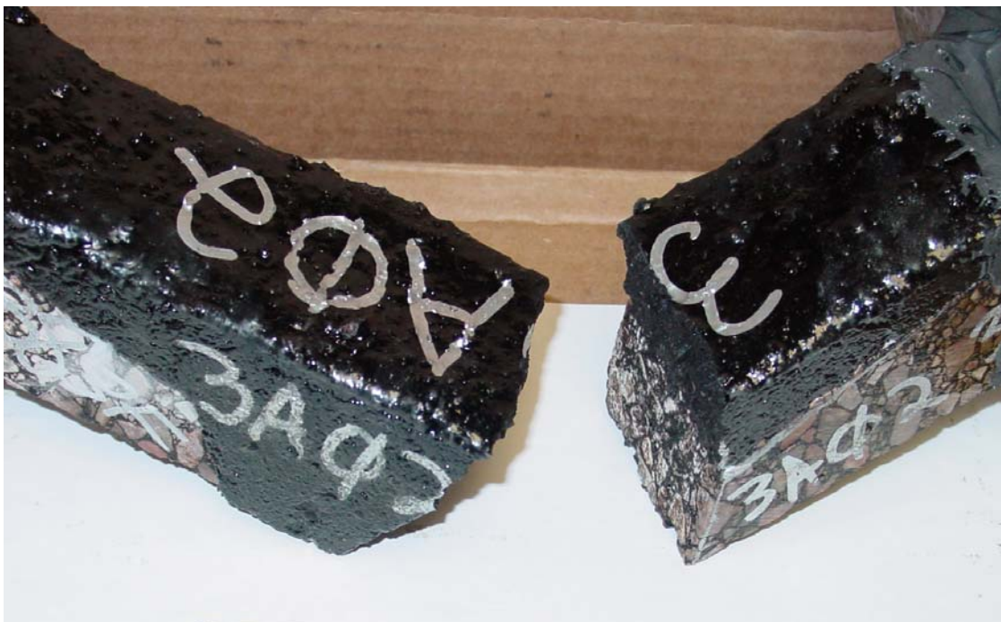
Figure 5.9 TSRST Tapered Overband Configuration Failure Mode for All Materials
