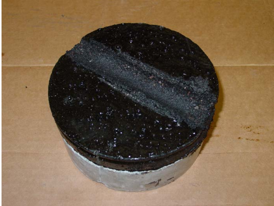
Figure 5.12 Rutting in Level & Go Crack Surfacing Material
