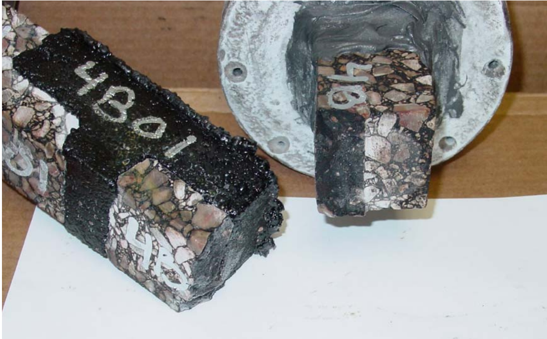
Figure 5.10 TSRST Mill & Fill Configuration Primary Failure Mode for All Materials
