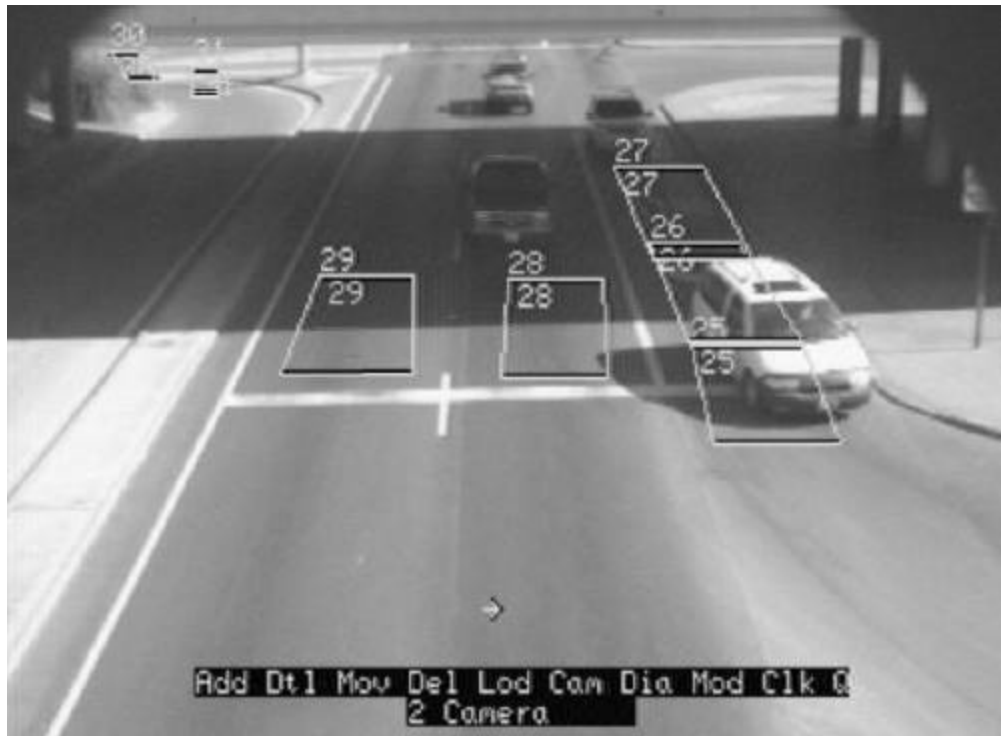
Figure 5.3: Shadows From Tall Vehicles and Bridge Structures Source: Video Detection for Intersection and Interchange Control (5-28)
