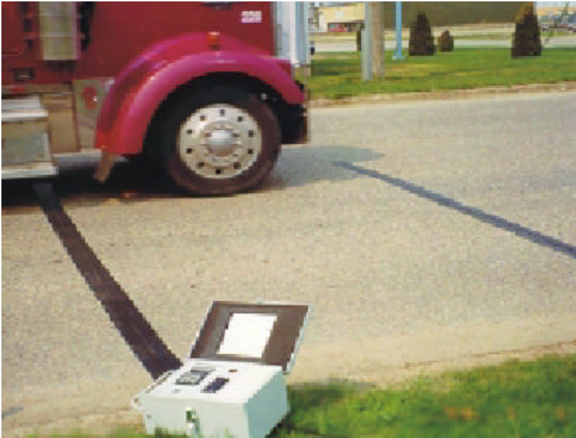
Figure 4.14: Typical Portable Fiber Optics Sensor Installation
