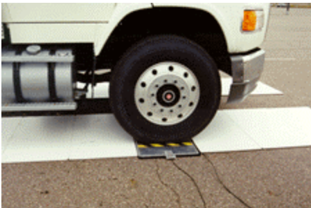
Figure 4.13: Truck Driving Over Portable Capacitive Mat WIM System
