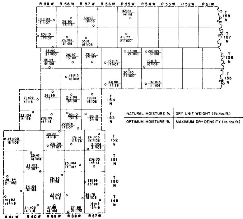
Figure 28. Map of Nelson and Walsh Counties showing values for four types of engineering data and the locations where such data was available.
