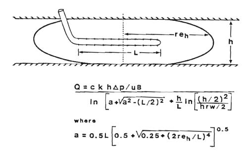
Figure 1. Comparison of vertical and horizontal well drainage volume schematic (Meridian Oil, Inc., North Dakota Industrial Commission Case #4606).
