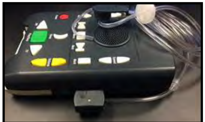
Breath Switch, shirt clip and mouth tube connected to DTBM.
